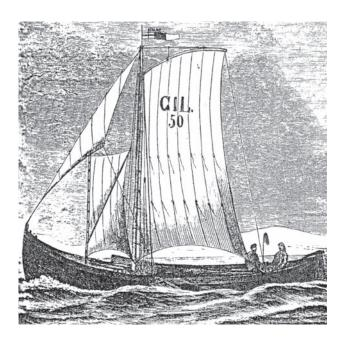
Typical fishing boat used on the Baltic lagoons – a Taglerpolten from the Oder Lagoon, Angelkhane from Vistula Lagoon and Kurrenkahn from Kurland Lagoon representing various forms of a local type of watercraft.
