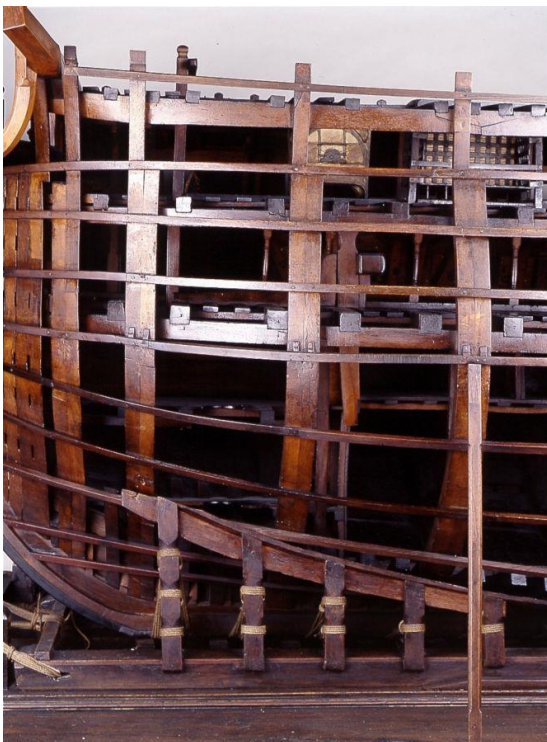
Image 20, Same details as in the previous image, but from the bow of the ship. Museo Naval de Madrid. Nº de inventario MNM 918.
