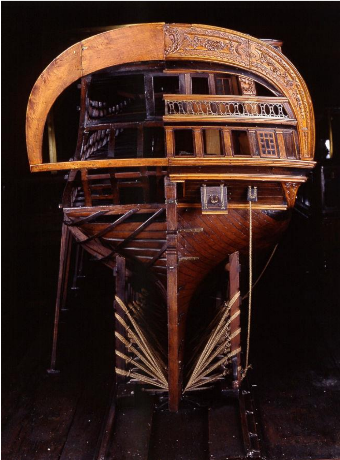
Image 17. Detail of the stern of the 74-gun ship with its ropes that pass from side to side. Museo Naval de Madrid. N° de inventario MNM 918.
