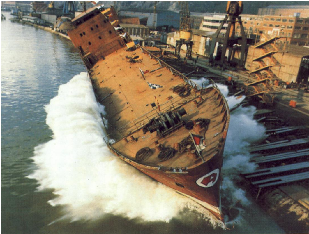
Image 1. Where the launching of a ship from the side is represented. On the right we can see the launch bed (La "BOTADURA": el nacimiento de un "BUQUE", 2020).
