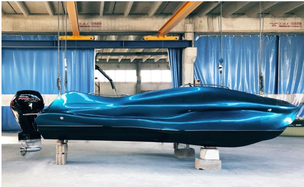
Image 29. MAMBO continuous fiber 3D printed boat by moi Composites ( 3dprintingmedia.network/3d-printing-boats-is-becoming-standard-practice )
