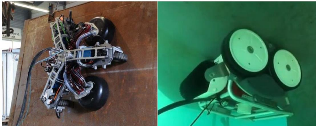
Image 15. On the left – ship keel cleaner produced by Fleet Cleaner Grijpskerk - The Netherlands, on the rights - ship keel cleaner produced by Hulltimo, France (BlueTech.eu, 2016)
