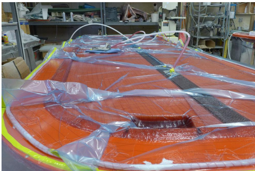
Image 8. You can see the core (with checkered appearance) in this part, about to be vacuum-bagged at Sabre Yachts (boats.com)
