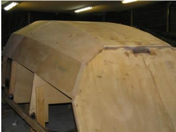
This Black Swan from Israel with most of the pre-shaped planks fitted - again the seams are to be epoxy/taped.
