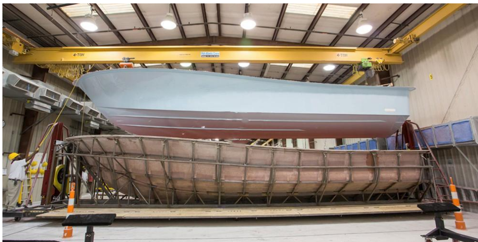
Image 6. Overhead cranes are often used to lift major boat parts, like this hull for a Regulator fishing boat, out of the molds and into position for further assembly (boats.com)
