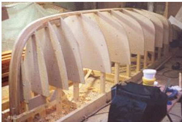
The chipboard moulds (sectional shapes) are carefully erected onto a simple wood strongback.
