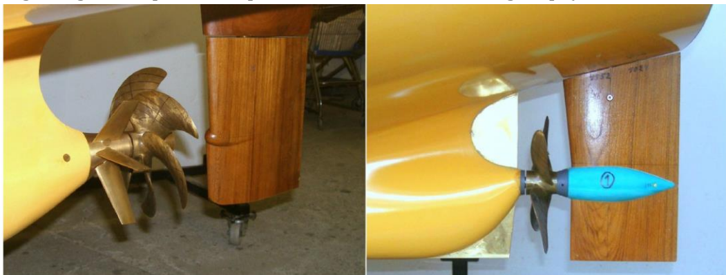
Image 9. Figure (on the left side) the stator pre-swirl developed by Daewoo Shipbuilding & Marine Engineering – South Korea, (on the right side) a system with a rudder bulb and an interceptor developed by Scandinavian study (HOLLENBACH, 2011).
