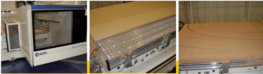
Image 26. The working process: a) CNC plant; b) wooden panel on the work surface; c) first cut along the lines (FRAGASSA C., 2016)
