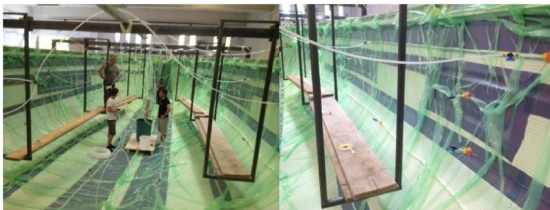
Image 19. Hull manufacturing with the infusion process at the Fano establishment (BlueTech.eu, 2016)
