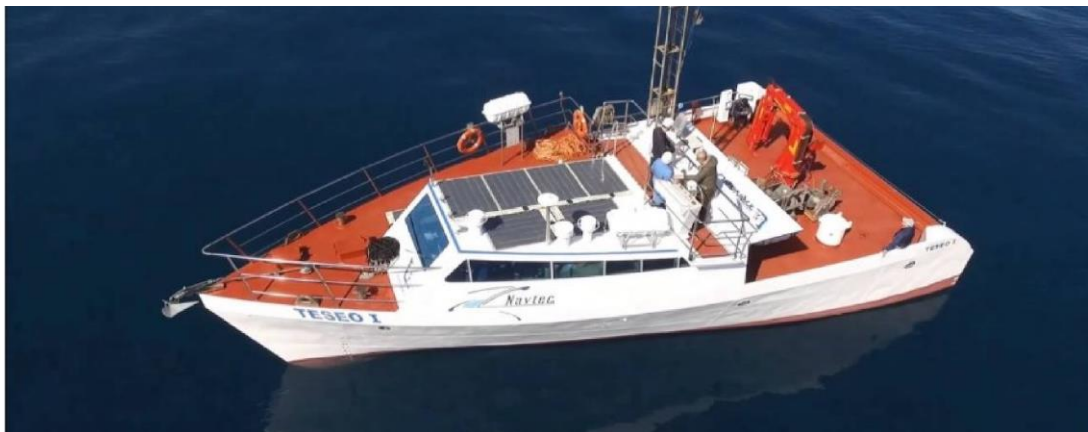
Image 13. Teseo I, the first hybrid commercial fishing vessel built by Cantiere navale Tringali6 (Augusta SR, Italy) in the framework of research project PON TESEO: High Efficiency Technologies for Energy and Environmental Sustainability On-board (BlueTech.eu, 2016)
