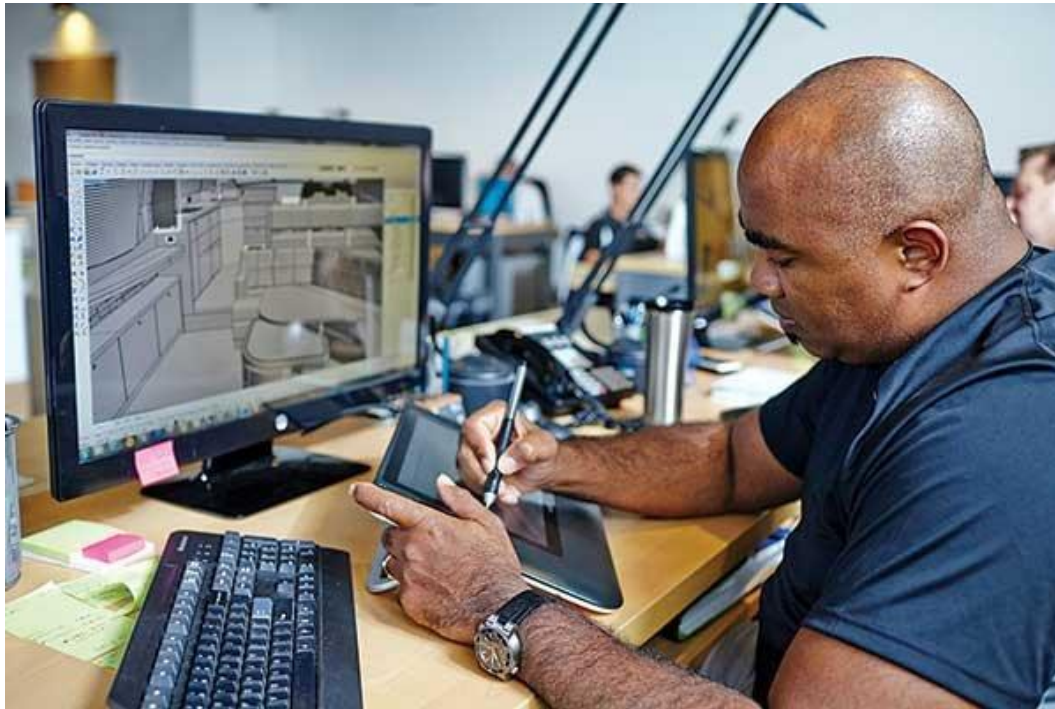
Image 25. Using CAD programs, designers achieve astonishing detail: colors and textures of upholstery and furniture, precise hose and wire runs, detailed systems installation. These instructions are sent directly to CNC routers to create the parts from which the final boat is assembled. Taken at Sea Ray (Boat U.S. Association, 2016).
